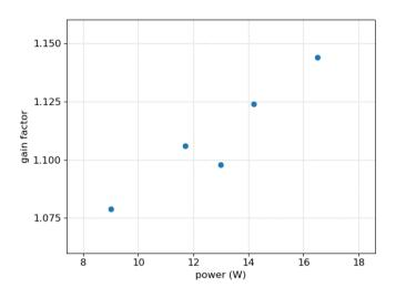
**Figure 8.** Chirping gain vs. laser power. The chirping frequency and chirping rate were 6 kHz and 0.78 MHz  $\mu$ s<sup>-1</sup> at an alt/az pointing of about 75°/210°. The measurements were taken consecutively over approximately 10 minutes during the night of Sep 18.
