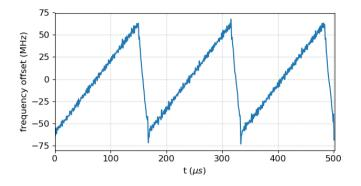
**Figure 3.** Frequency of the laser during chirping. In this case, the chirping frequency was 6 kHz and the chirping peak-to-peak amplitude was 120 MHz. The y-axis shows the offset from the  $D_2$  line centre frequency.
