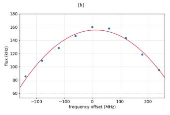
**Figure 4.** Measured return flux for an un-chirped laser. The true centre of the Boltzmann distribution is offset by +15 MHz from the centre frequency of the laser.
