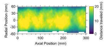
FIG. 6. Distance travelled as a function of the starting position for an inner drum diameter of 140 mm. The particles used were ballotini with a diameter of 1.0 - 1.3 mm. The drum rotated at 0.066 rpm and was filled to a fill level of 25 %.
