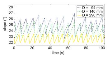
FIG. 2. The slope of the free surface as a function of time for three drum diameters: 94 mm (dotted blue), 140 mm (dashed red) and 290 mm (yellow) rotating at 0.066 rpm and a fill level of 25 %. The particles are ballotini with a diameter of 1.0 - 1.3 mm.
