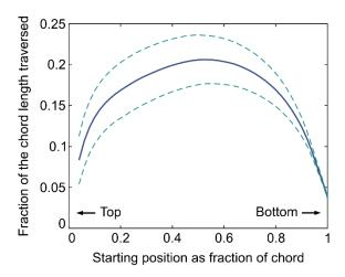
FIG. 7. Mean fraction of the chord length travelled as a function of the starting position along the chord. The data has been averaged from 16 avalanches and the dashed lines show one standard deviation. The cylinder has a diameter of 300 mm and rotates at 0.066 rpm. The fill level is 25 % and the particles are glass ballotini with a diameter of 1.0 - 1.3 mm.
