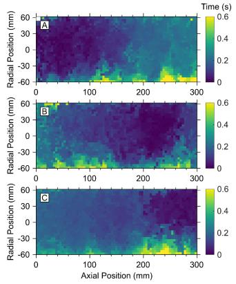
FIG. 3. Local avalanche initiation time shown for three independent avalanche events. The color indicates the time after the start of the avalanche for which the velocity at a point on the free surface exceeds 3 mm/s. The cylinder has an internal diameter of 140 mm and rotates at 0.066 rpm. The fill level is 25 % and the particles are glass ballotini with a diameter 1.0 - 1.3 mm.
