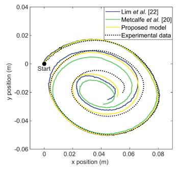
FIG. SI 1. The pink particles' change in center of mass during two drum rotations is shown. We compare our proposed model and experimental data with the models of Lim et al. [22] and Metcalfe et al. [20]. The positions are given relative to the starting point.
