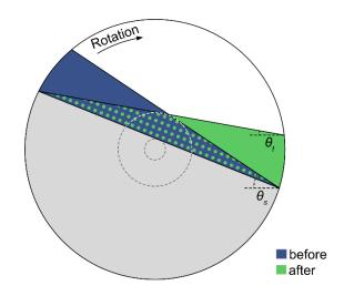
FIG. 1. Geometric models of an avalanche where  $\theta_s$  is the angle between the bed surface and the horizontal before an avalanche and  $\theta_t$  is the corresponding angle after an avalanche: the model proposed by Metcalfe et~al. [20] has the purely blue wedge falling down to the purely green wedge. The model proposed by Lim et~al. [22] starts width a wedge made of all areas containing blue falling down to the wedge of fully green plus green spotted.
