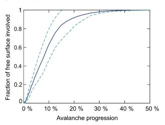
FIG. 4. The fraction of the bed surface involved in an avalanching event as a function of the fraction of the duration of an avalanche event. The mean and standard deviation were calculated from the data of 20 avalanches. The cylinder has a diameter of 140 mm and rotates at 0.066 rpm. The fill level is 25 % and the particles are glass ballotini have a diameter of 1.0 - 1.3 mm.
