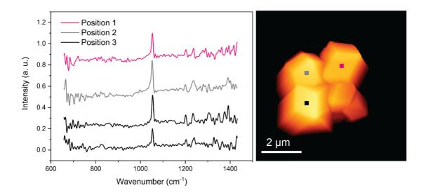
FIG S5: Local nanoFTIR spectra measured on individual ZIF-71 crystals reveal chemical homogeneity.
