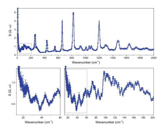
FIG S1: Inelastic neutron scattering (INS) data with error bars for a powder sample of ZIF-71.
