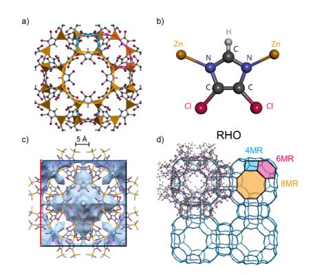
FIG 1: Framework structures of ZIF-71: a) ZIF-71 unit cell where the inorganic building blocks are illustrated by the ZnN<sub>4</sub> tetrahedra. b) The building unit showing the Zn–dcIM–Zn linkages. c) The blue surfaces denote the nanopore, corresponding to the solvent accessible volume within the open framework structure. d) Illustration of the RHO topology, highlighting the apertures of the 4-, 6-, and 8-membered rings (MR).
