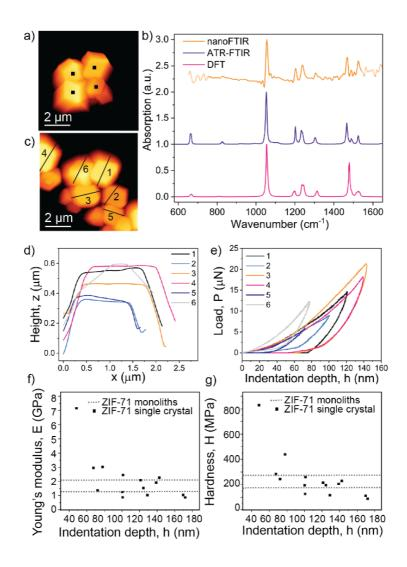
FIG 4. Nanoscale analytics of ZIF-71 single crystals. a) AFM image of ZIF-71 crystals with indicated positions for nanoFTIR measurements. b) Corresponding nanoFTIR spectra
