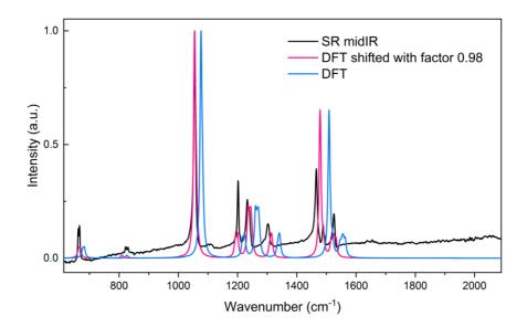
FIG S3: Bulk shift of DFT simulated spectrum versus the experimental mid-IR spectrum of ZIF-71.
