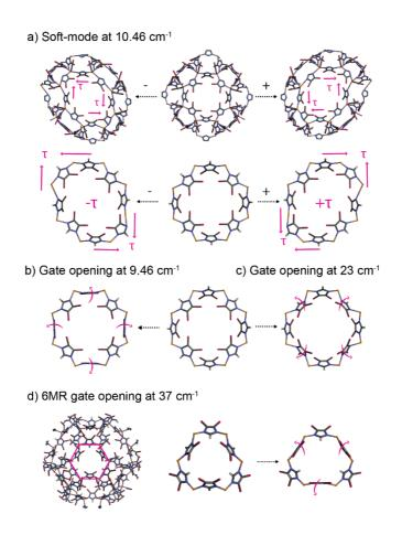
FIG 3: Low-energy lattice modes of ZIF-71. a) Soft mode caused by a shear deformation of the 8MR. b, c) Gate-opening mechanisms of the 8-membered ring (MR) *via* synchronous rocking of opposite organic linkers. Pink arrows designate the collective dynamics affecting the geometry of pore cavity. d) Gate-opening of the 6MR through synchronous flapping of the linker units.
