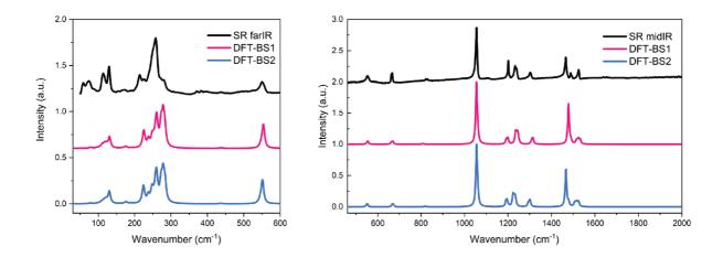
FIG S2: Comparison between infrared spectra of ZIF-71 obtained from synchrotron-radiation (SR) far-IR experiments and DFT simulations employing two different basis sets (BS1 and BS2).
