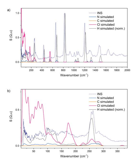
FIG S4: INS spectra derived from the phonon calculation compared with experimental measurement. No shift was applied, but the simulated spectrum for hydrogen (H) has been scaled down (normalization between 0 and 1) for better visualization.
