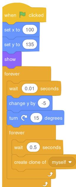
Figure 3: Example of a *Forever Inside Loop* bug pattern, taken from a publicly shared project: The blocks in the outer forever-loop will only be executed once, since the execution will not leave the inner forever-loop.
