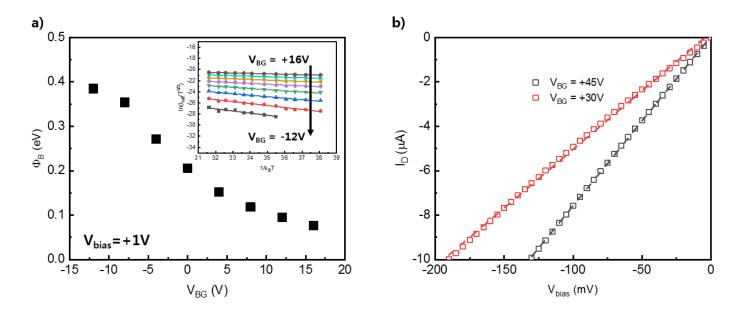
Figure. S4 (a) Arrhenius plot in reverse bias regime (inset) and Schottky barrier heights obtained in this study,(b) current versus bias voltage characteristic in the linear non-diode regime.
