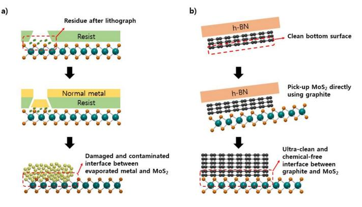
**Figure. S3 Comparison between direct metal deposition and 2D metal contacts:** (a) standard lithography and metal evaporation process and (b) 2D vdW metal contact process.
