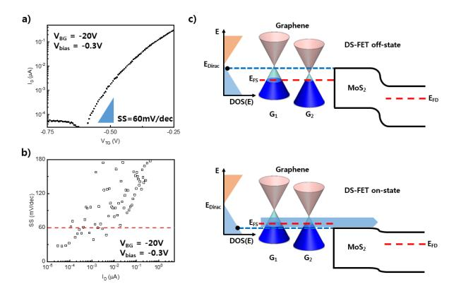
Figure S8. MoS<sub>2</sub> DS-FET measurement and its band diagram. a, b Transfer curves of the DS-FET at  $V_{BG}$ = -20 V and  $V_{bias}$  = -0.3 V. c Band diagrams of DS-FET. As the top-gate voltage,  $V_{TG}$ , is applied to the MoS<sub>2</sub> channel, the injection current density increases.
