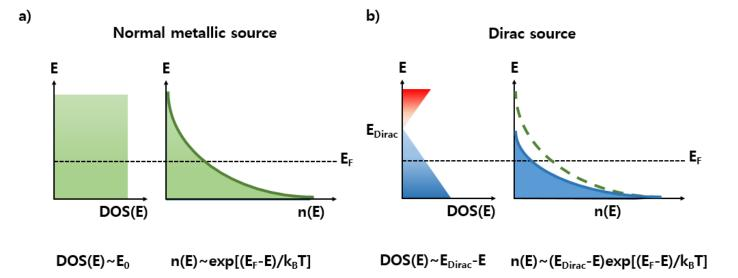
Figure. S1 State and electron densities of (a) normal metallic and (b) Dirac sources.
