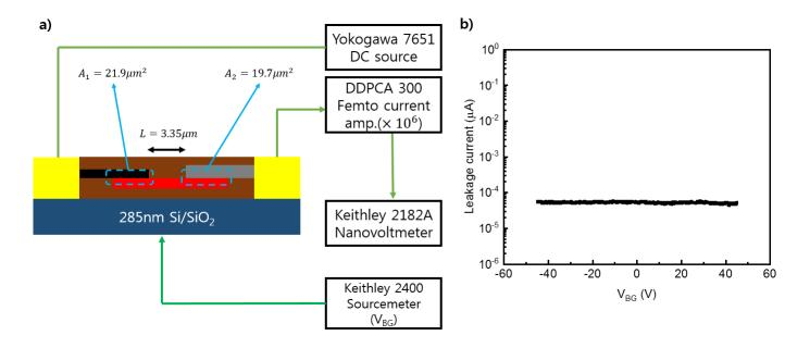
Figure. S9 (a) Specified device dimension as well as measurement setup and (b) system leakage level observed in this study. In (a), red, black, gray, brown, and yellow colors denote  $MoS_2$ , graphene, graphite, h-BN, and contact metal (Cr/Au = 5/60-nm-thick), respectively.
