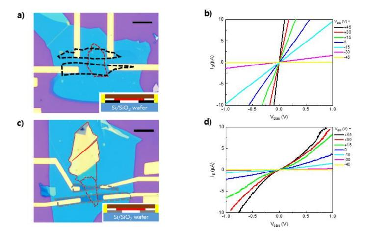
Figure. S6 Optical images of (a) graphene–MoS<sub>2</sub>–graphene and (c) graphite–MoS<sub>2</sub>–graphite interfaces along with corresponding transfer curves—(b) and (d), respectively. In (a) and (c), the black, gray, brown, red, and yellow colors represent graphene, graphite, h-BN, MoS<sub>2</sub>, and contact metal (Cr/Au), respectively. Scale bar, 10µm.
