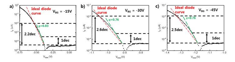
Figure 3. Slopes of DS Schottky diode versus ideal diode and recorded ideality factor in 2D vdW material-based diode. Comparison of slopes between the proposed DS Schottky diode and an ideal diode. Black and red dotted data represent those of the DS Schottky diode and an ideal diode, respectively. The DS Schottky diode exhibits an average  $\eta$  of 1 for 2.2, 2.6, and 2.5 decades when  $V_{BG} = -15$ , -30, and -45 V, respectively.
