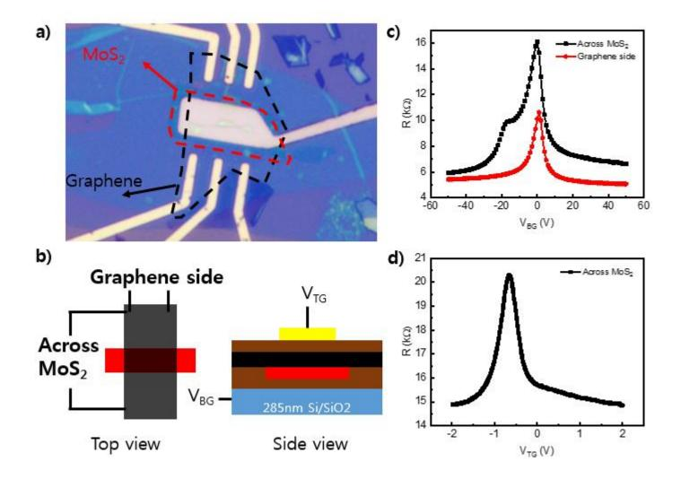
**Figure. S5 (a)** Image of the test device and (**b**) its schematic. Si acts as a global back gate, and the top gate is designed to gate the overlapping region of  $MoS_2$  and graphene exclusively. In (**b**), the black, brown, and red colors indicate graphene, hBN, and  $MoS_2$  respectively. (**c**) Two-probe "across  $MoS_2$ " (black) and "graphene side" (red) measurements performed considering a Si back gate. (**d**) Two-probe "across  $MoS_2$ " measurement considering top gate.
