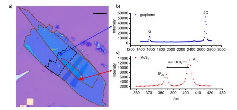
**Figure. S10** (a) Optical image of graphene– $MoS_2$ –graphite heterojunction device. The blue and red dots indicate the positions of the graphene and  $MoS_2$  Raman spectra measurements, respectively. Scale bar, 10µm. (b) Raman spectra of graphene, and (c) Raman spectra of  $MoS_2$ .
