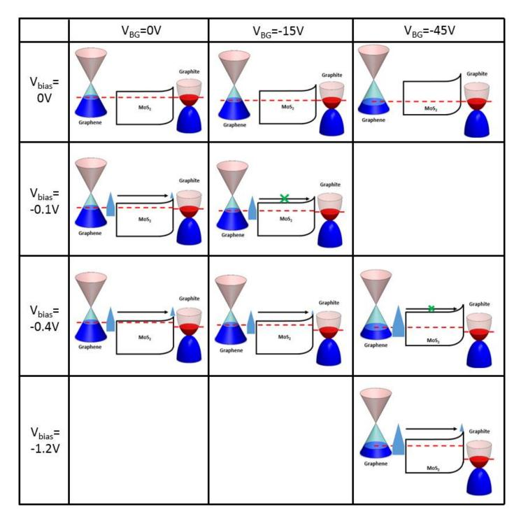
Figure S11 Band diagrams in diode regime.
