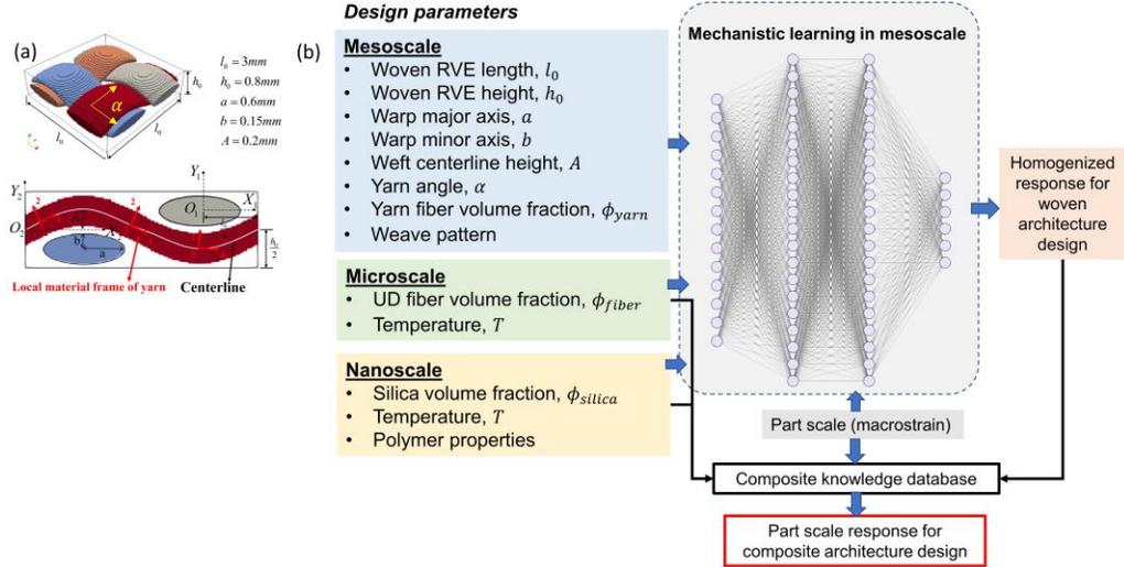
Fig 8. (a) Woven composite and RVE and design parameters, (b) design parameters of composites at multiscale and composite knowledge database preparation for system and design.
