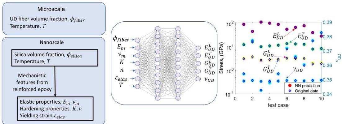
Fig. 7. (a) Mechanistic learning in microscale UD composite using a feed-forward neural network, (b) accuracy of neural network prediction for the elastic constants of the UD composites.
