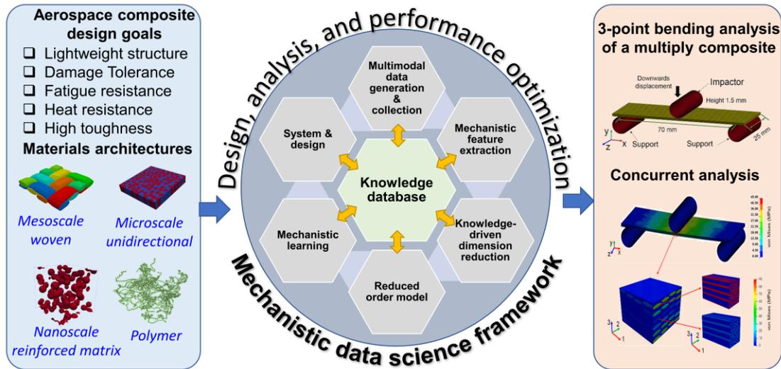
**Fig 2.** Mechanistic data science framework and its six components to create knowledge database for composite design, analysis and performance optimization.
