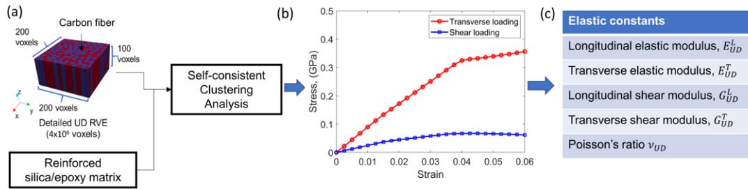
Fig 6. (a) Workflow for generating stress-strain curve using Self-consistent Clustering Analysis (SCA) method, (b) stress-strain response for transverse and shear loading of unidirectional composite with 50% fiber volume fraction and 15% silica reinforcement in the matrix, (c) extracted features from the stress-strain curve.
