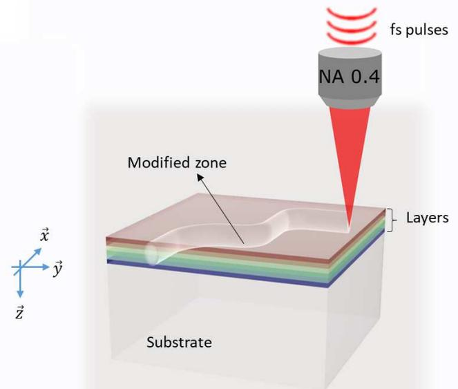
Figure 1. Working principle of multi-layer ultrafast laser modification. A substrate with a stack of thin transparent films (each thinner than the laser-wavelength) is exposed to a femtosecond laser to induce local intermixing and phase transitions in the material, following an arbitrary trajectory.
