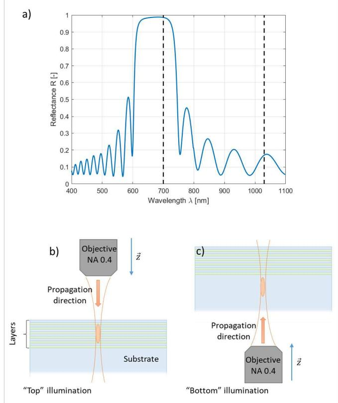
Figure 2. a) Reflectance spectra of the samples. 700 and 1030 nm wavelengths positions are marked with black dashed lines. b) and c) illustrate the two exposure modalities explored in this work: the "top" illumination and the "bottom" illumination (through the substrate) of the layer stack, respectively.
