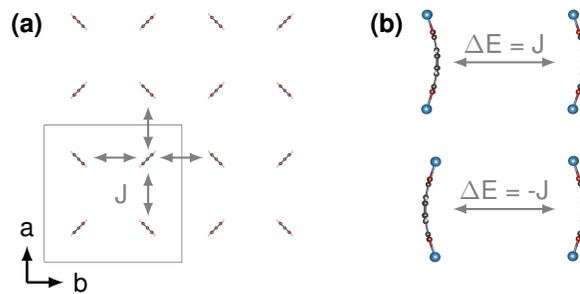
FIG. 2. Exchange interaction of buckled linker molecules. (a) shows the molecular arrangement of BDC linker molecules in MOF-5 in the  $\mathbf{a} - \mathbf{b}$  plane. Molecules form the pattern of a square lattice. (b) Shows the energy difference between ferro- and antiferro-buckling.
