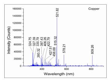
Figure 2: LIBS spectrum of copper acquired with linearly polarized laser light.
