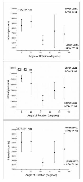
**Figure 5**: Variation in intensities of atomic emission lines in LIBS spectra of Cu with change in the polarization state of the excitation laser beam.
