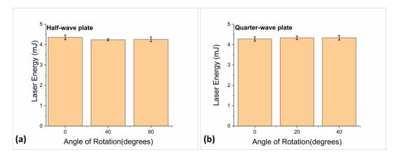
**Figure 8**: Variations in laser energy at different orientations of the (a) half-wave plate and (b) quarter-wave plate.
