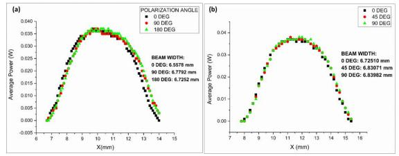
**Figure 7**: Laser beam profile in the presence of (a) half-wave plate at different orientations and (b) quarter-wave plate at different orientations.
