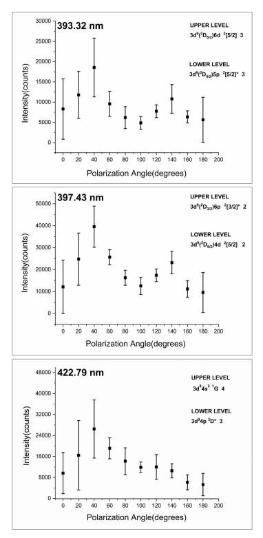
**Figure 4**: Variation in absolute intensities of ionic emission lines in LIBS spectra of copper with respect to the polarization direction of the linearly polarized excitation laser beam.
