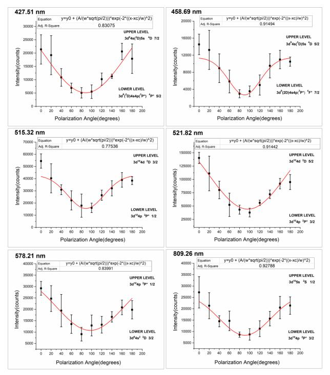
**Figure 3**: Variation in intensities of atomic emission lines in LIBS spectra of copper as a function of polarization direction of a linearly polarized excitation laser beam (all data fitted to Gauss function with equations indicated in each panel).
