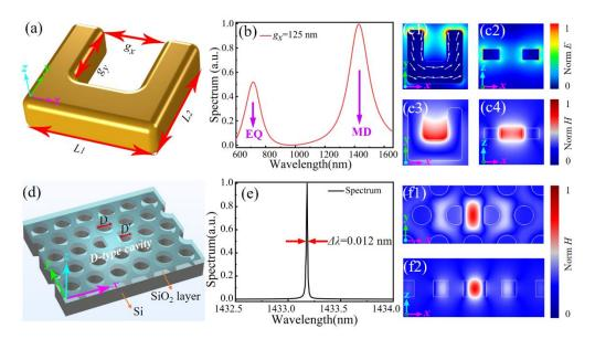
**Figure 1.** (a) Schematic of a gold SRR with defined geometric parameters. (b) Calculated scattering spectrum of an individual SRR showing EQ and MD resonant modes. (c1, c2) Electric field and (c3, c4) magnetic field distributions of SRR at the resonant wavelength of 1430 nm. (d) Schematic of the D-type PCNC with D' = 0.8 D. (e) Calculated scattering spectrum of the D-type PCNC. (f1, f2) Magnetic field distributions of D-type PCNC at *x*-*y* and *x*-*z* cross-sections, respectively.
