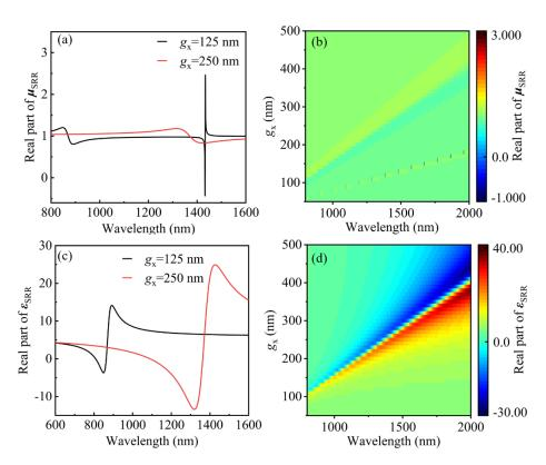
**Figure 2.** (a) The real part of the retrieved effective permeability  $\mu$  around the plasmon resonant of single SRR. (b) The  $\mu$  distribution about the  $g_x$  size of SRR from 50 to 500 nm. (c) The real part of the retrieved effective permittivity  $\varepsilon$  around the plasmon resonant of single SRR. (b) The  $\varepsilon$  distribution with the  $g_x$  size of SRR from 50 to 500 nm.
