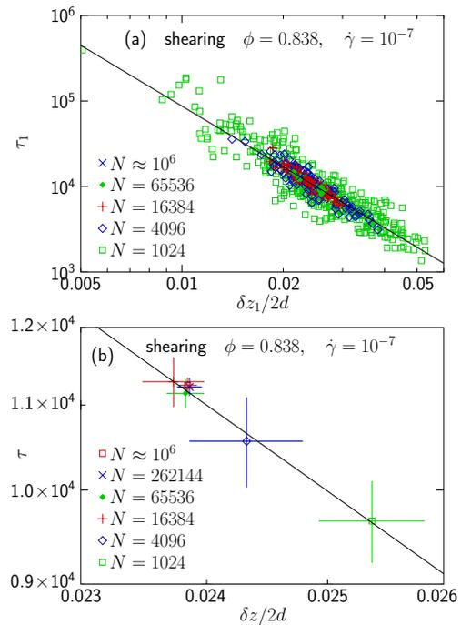
FIG. 7. Relaxation time versus contact deficiency,  $\delta$ , for the shearing case and different system sizes,  $N = 1024$  through  $\approx 10^6$ . Panel (a) shows individual measurements together with the line with slope  $-b$ , where  $b = 2.36$ . Panel (b) shows  $\tau$  vs  $\delta z$ , which are the geometric averages of the same quantities. This panel shows clearly that the finite size effects are small and unproblematic for the shearing case.
