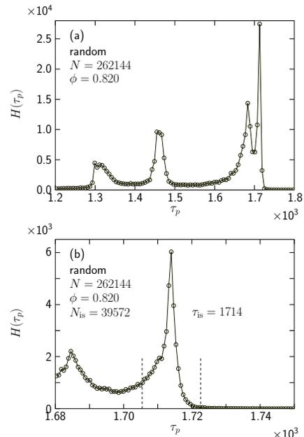
FIG. 10. Determination of  $\tau_{is}$  and the size of the island,  $N_{is}$ , which is the number of particles that belong to the corresponding peak in the histogram. Panel (a) shows the complete histogram and panel (b) is a zoom in on the uppermost peak.  $N_{is}$  is the number of particles with  $\tau_p$  in the interval  $\tau_{is} \pm 0.5\%$ .
