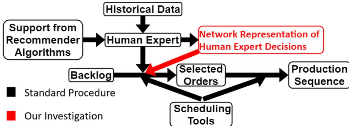
Figure 1: Flow chart illustrating how the steel planning process could profit from our network method.
