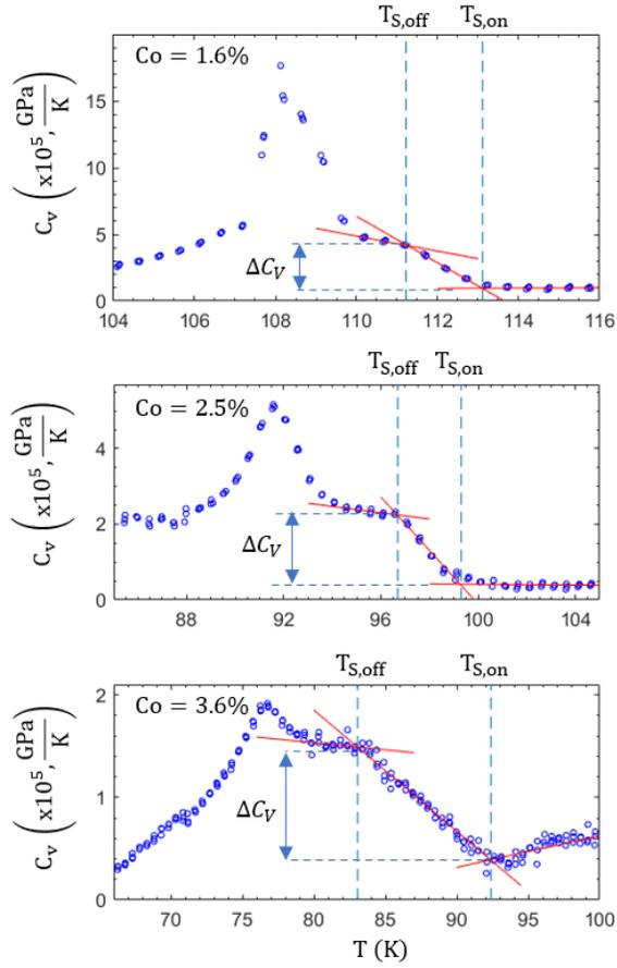
FIG. 3. Heat capacity  $C_V$  with background phonon contribution subtracted for 3 doping values. The step-like increase  $\Delta C_V = C_V(T_{S,off}) - C_V(T_{S,on})$  is defined from the difference between intersecting linear fits at the jump onset ( $T_{S,on}$ ) and flattening ( $T_{S,off}$ ) of the heat capacity. Extracted values of  $\frac{\Delta C_V}{T_S}$  across the doping phase diagram presented in Fig. 4.
