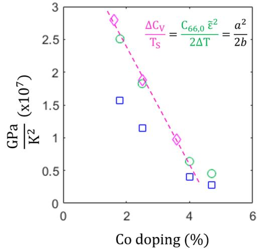
FIG. 4. Comparison of the thermally-normalized heat capacity discontinuity  $\frac{\Delta C_V}{T_S}$  and the lattice quantity ratio  $\frac{C_{66,0} \tilde{\epsilon}^2}{2 \Delta T}$  determined from either  $\Delta T = 25$  (green) or  $\Delta T = 40$  (blue) (see main text). Line is a guide to the eye.
