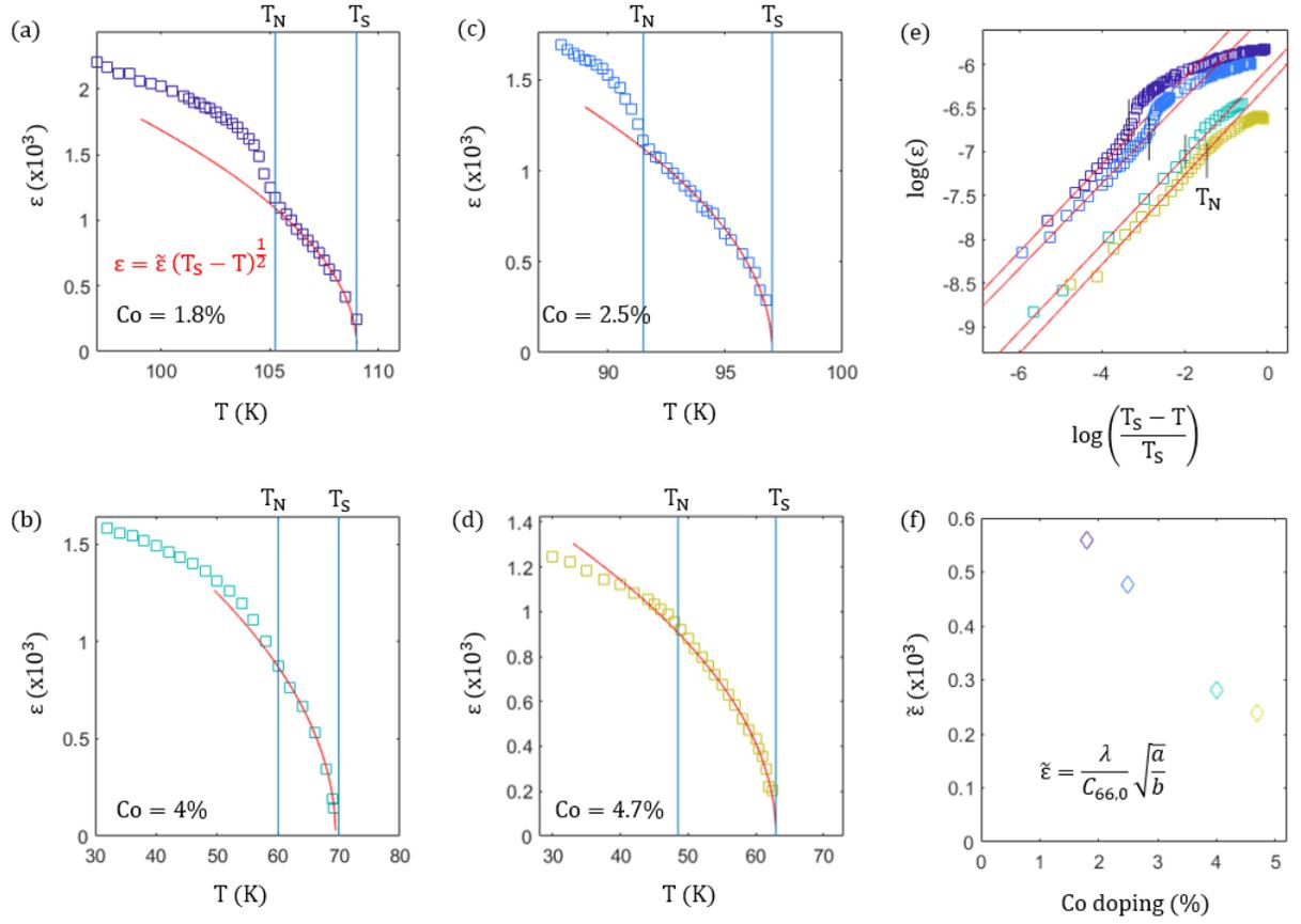
FIG. 1. (a-d) Spontaneous orthorhombicity for 4 Co-dopings. Red line is a mean-field fit  $\varepsilon_S = \tilde{\xi}(T_S - T)^{\frac{1}{2}}$  within the nematic phase ( $T_N < T < T_S$ ). (e) Same dopings on log-log scale plotted vs reduced temperature. (f) Magnitude of orthorhombicity vs doping.
