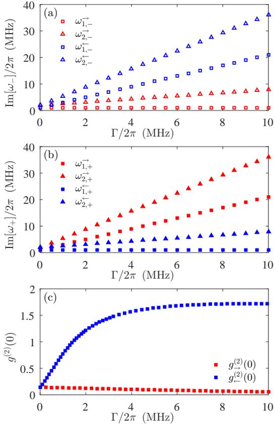
FIG. 4. Imaginary parts (a)  $\text{Im}[\omega_{n,-}]$  and (b)  $\text{Im}[\omega_{n,+}]$  of the bidirectional eigenvalues  $\omega_{n,\pm}$  ( $n = 1, 2$ ) versus the dissipative coupling  $\Gamma/2\pi$ . (c) Bidirectional correlation function  $g^{(2)}(0)$  versus  $\Gamma/2\pi$  with  $\Delta/2\pi = 10$  MHz. Other parameters are the same as in Fig. 2.
