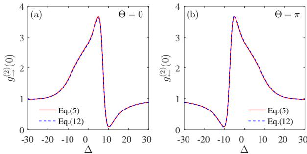
FIG. 5. Comparison of the second-order correlation function  $g_{\pm}^{(2)}(0)$  for the cases with and without the coupling between the cavity and the waveguide, which are calculated using Eq.(5) and Eq.(12). In (a) and (b), the drivings are loaded via port 1 and port 2, respectively. The newly introduced parameters are chosen as  $\beta_{\text{in}}/2\pi = 1$  MHz and  $\zeta = 1$ , while other parameters are the same as in Fig. 2(c).
