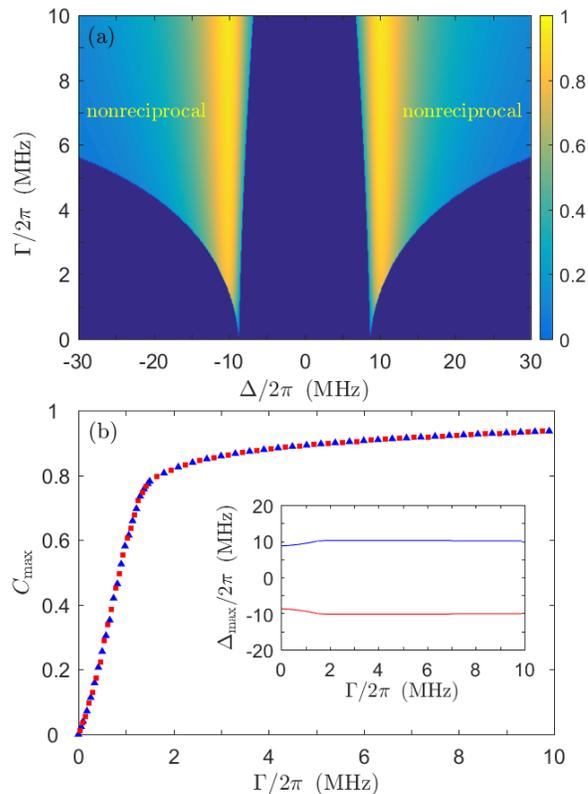
FIG. 3. (a) Dependence of the bidirectional contrast ratio  $C$  on the dissipative coupling strength  $\Gamma/2\pi$  and the detuning  $\Delta/2\pi$ . (b) The maximized contrast ratio  $C_{\text{max}}$  versus the dissipative coupling strength  $\Gamma/2\pi$ , with the corresponding detuning  $\Delta_{\text{max}}/2\pi$  of blue triangles (red squares) indicated by the blue (red) curve in the inset. Other parameters are the same as in Fig. 2.
