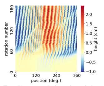
Fig. 4. The space-time plot showing the growth of a ripple pattern produced from the horizontally flat surface by  $v_{\rm ap} = 0.78 \text{ m s}^{-1}$ .
