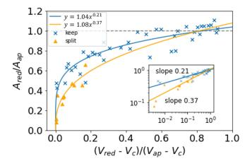
Fig. 8. Amplitude ratio versus normalized velocity. The different behaviors can be confirmed between the keep type (cross marks) and split type (triangle marks). Solid blue and yellow curves are the fitting to keep and split types, respectively. The inset shows the double logarithmic plot of the same data.
