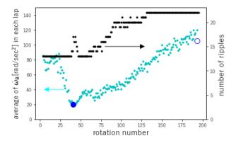
Fig. 10. The average angular acceleration at the bottom,  $\dot{\omega}_{\rm B}$ , is plotted by green dots and the number of ripples is shown by black dots. A blue filled circle and a blue empty circle indicate the minimum and final values of  $\dot{\omega}_{\rm B}$ , respectively.
