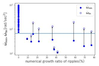
Fig. 11. Filled circles show  $\dot{\omega}_{\min}$  in both keep and split types. There seems a threshold value (65 rad s<sup>-2</sup>) as shown by the horizontal line. Empty circles show the final values  $\dot{\omega}_{\text{fin}}$  in the split type. Most of them exceed the threshold level.
