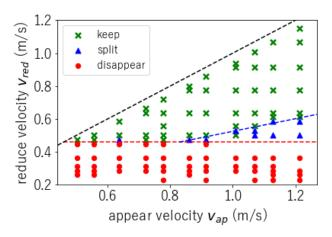
**Fig. 6.** The phase diagram of the ripples variation with various combinations of  $v_{\rm ap}$  and  $v_{\rm red}$ . The black dashed line represents  $v_{\rm red} = v_{\rm ap}$ . The red and the blue dashed lines are drawn to represent the boundaries of the phases.
