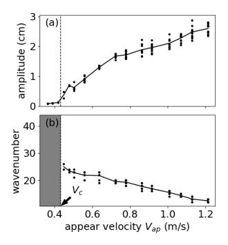
Fig. 3. (a) Average amplitude and (b) wavenumber of the ripples developed on the granular surface with  $v_{\rm ap}$ . Each symbol indicates individual experimental result. Solid lines connect the average values of the same  $v_{\rm ap}$  data. The region below the critical velocity  $v_{\rm c} = 0.43$  m s<sup>-1</sup> is shaded grey in (b).
