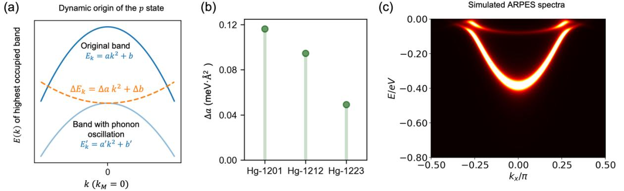
**Figure 3. ARPES simulation using the 3-band model.** (a) Illustration of the origin of the heavy flux state from the dynamic change of the highest occupied band around the  $k$ -point  $(0.5, 0.5, 0)$  perturbed by phonons. (b)  $\Delta\alpha$  of the three Hg-family materials from an average over the last four phonon modes from DFT simulations. (c) Simulated ARPES spectra with  $k_y = 0.85\pi$ .
