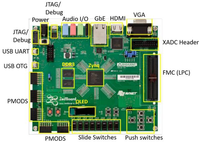
FIG. 5. The Xilinx Zynq FPGA and its components.
