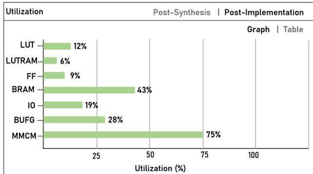
FIG. 3. Device Utilization for Zynq FPGA
