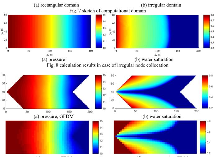
(c) pressure, FDM (d) water saturation, FDM Fig. 9 Comparisons of the calculation results at the 250<sup>th</sup> day in case of irregular boundary shape
