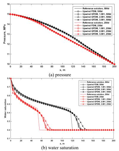
Fig. 4 Comparison of calculation results of oil-phase pressure and water saturation on y = 40m section
