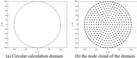
Fig. 2 sketches of a circular domain and a corresponding node cloud
