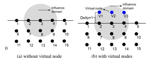
Fig. 10 sketches of the allocation nodes in the influence domain of the boundary node 3
