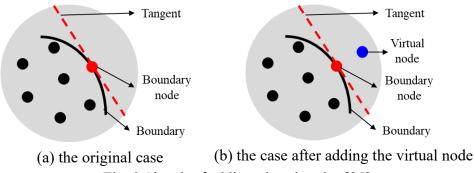
Fig. 3 Sketch of adding virtual nodes [25]
