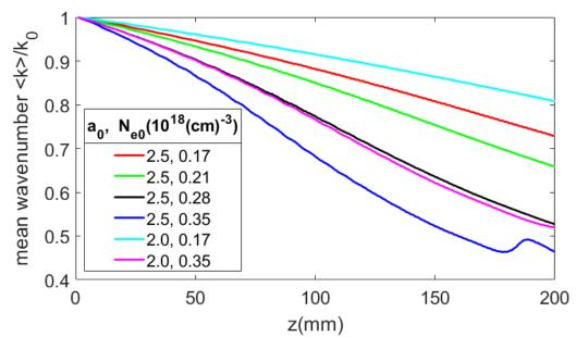
**Figure C3.** Mean normalized wavenumber  $\langle k \rangle / k_0$  of the laser pulse along the plasma waveguide.
