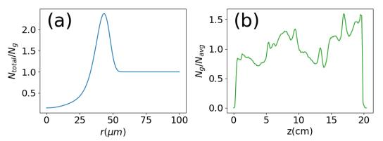
Figure C2. (a) Transverse plasma density profile (where  $N_{tot}(r) = N_e(r)$  for a fully ionized profile) and (b) measured longitudinal gas density profile of the gas jet (3mm profile from Fig. 1(c)), where  $N_{avg}$  is the axial average gas density.
