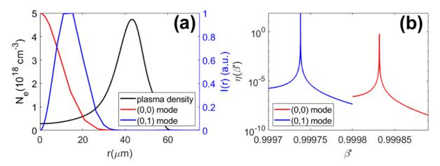
Figure B1. (a) Calculated (p, m) = (0,0) and (0,1) modes calculated for waveguide of Fig. 1(g)(ii) with  $N_{e0} = 3.2 \times 10^{17}$  cm<sup>-3</sup>. (b) Plots of  $\eta(\beta')$  vs.  $\beta'$  showing the resonances corresponding to the (0,0) and (0, 1) modes.
