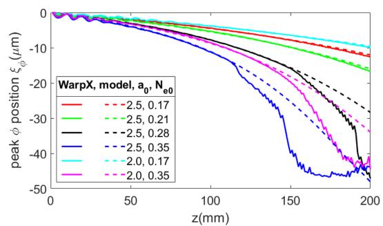
**Figure C4.** Position  $\xi$  of the peak potential of the plasma wake bucket following the laser pulse in a frame moving at the group velocity  $v_{g0}$  of the undepleted laser pulse. The reduced plasma wave phase velocity effectively shortens the LWFA dephasing length. Solid curves: WarpX simulation. Dashed curves: model fit.
