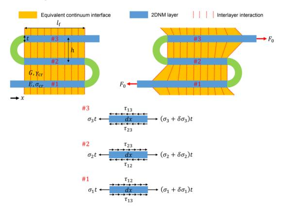
Fig. 2 Schematic illustrations of the theoretical model for self-folded two-dimensional nanomaterials (SF-2DNMs). A representative volume element (RVE) with a basic tri-folded configuration is adopted in our model. The interlayer interaction is represented by an equivalent continuum layer. The three folded 2DNM layers are marked as #1, #2 and #3. The material
