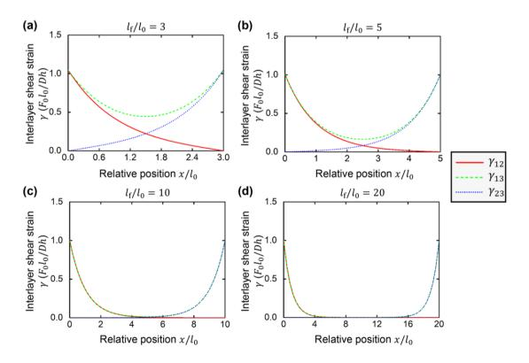
Fig. 4 Distributions of interlayer shear strain in self-folded two-dimensional nanomaterials
