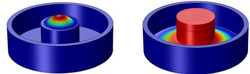
FIG. 5. Lowest order vibration modes for the sample holder. A COMSOL Multiphysics simulation gives an eigenfrequency of 70 kHz and 7 kHz for the (0, 1) drum mode for the center and outer platform, respectively from left to right.
