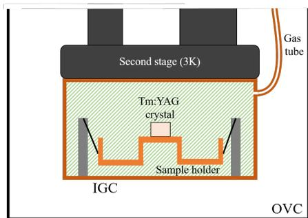
FIG. 1. Schematic cryostat cold part in configurations (b) and (c): the holder is suspended to the posts and the IGC is filled with helium gas. In configuration (a) the sample holder rests at the bottom of the IGC. (OVC: outer vacuum chamber. IGC: inner gas chamber.). The IGC and OVC are equipped with optical windows (not shown). A copper radiation shield (wrapped with multi-layer insulation), not represented for simplicity, is attached to the first stage.
