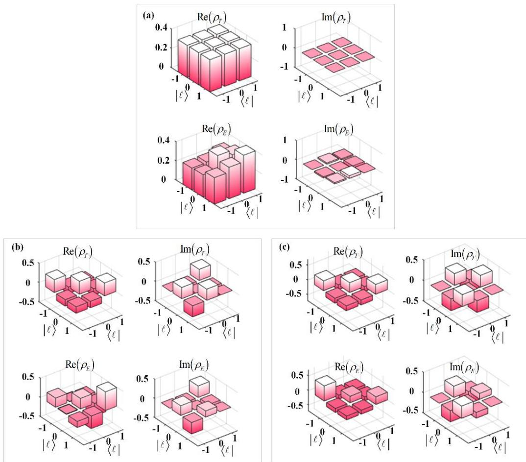
**Fig. 2 | Density matrices for 3-dimensional OAM teleportation,  $|\varphi_4\rangle_a = (|-1\rangle_a + |0\rangle_a + |1\rangle_a)/\sqrt{3}$ , conditional on three specific HDBSMs: (a)  $|\psi_{00}\rangle_{ab}$ , (b)  $|\psi_{01}\rangle_{ab}$  and (c)  $|\psi_{02}\rangle_{ab}$ . In each case, the upper rows are the original real and imaginary parts while the bottom are the experimental results.**
