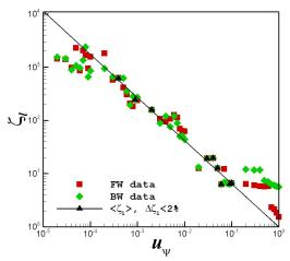
FIGURE 12. The scaling of the loss-time  $\zeta_l$  with the velocity  $u_{\psi}$  for the third turnstile. Color code: Red squares = the loss time for the forward lines, Green diamonds = the loss-time for the backward lines, Black triangles = the average loss-time  $\langle \zeta_l \rangle$  when the deviation of loss-times from exact equality  $\delta \zeta_l < 2\%$ . The loss-time  $\zeta_l$  scales as  $1/u_{\psi}^{0.8115}$ , giving the probability exponent  $d_3 = 4.3058$ .
