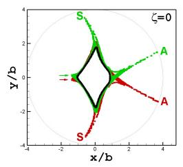
FIGURE 4. The magnetic turnstiles of the nonresonant stellarator divertor in the poloidal plane  $\zeta=0$ . Color code: Black = the outermost surface, Red = forward trajectories, Green = backward trajectories, Grey = the wall at r/b=4. The labels A and S denote the adjoining turnstile and the separated turnstile, respectively. The arrows show the pseudo-turnstile.
