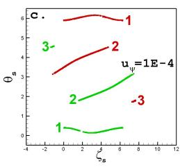
FIGURE 8. Footprints of the field lines with different velocities. The footprints of the first, second, and the third turnstile are labelled 1, 2, and 3, respectively. Footprints of the outgoing tubes are shown in red, and the incoming tubes are shown in green. (a)  $u_{\psi} = 1$ , (b)  $u_{\psi} = 10^{-2}$ , and (c)  $u_{\psi} = 10^{-4}$ .
