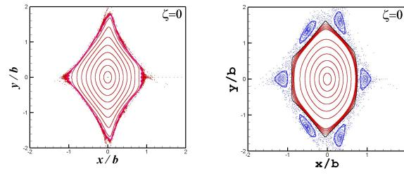
Figure 2. The Poincaré surface of section in the  $\zeta = 0$  poloidal plane for the magnetic field line trajectories in
