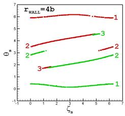
Figure 17. The magnetic footprints of the outgoing and the incoming tubes of all the three turnstiles on the wall  $r_{WALL} = 4b$ . Color code: Red = the footprints of the outgoing tubes, Green = the footprints of the incoming tubes. The labels 1, 2, and 3 denote the 1<sup>st</sup>, the 2<sup>nd</sup>, and the 3<sup>rd</sup> turnstile, respectively.
