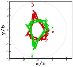
Figure 16. The  $3^{\rm rd}$  turnstile in the stellarator symmetric poloidal planes  $\zeta=75$  degrees for the outgoing tube, and in the  $\zeta=225$  degrees for the incoming tube. Color code: Red = the outgoing tube, Green = the incoming tube, Grey = the wall  $r_{WALL}=4b$ .
