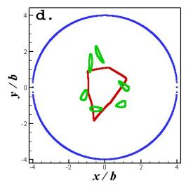
FIGURE 5. (a) The phase portrait in the  $\zeta = 0$  poloidal plane of a single period in the stellarator with a hybrid divertor. The good magnetic surfaces
