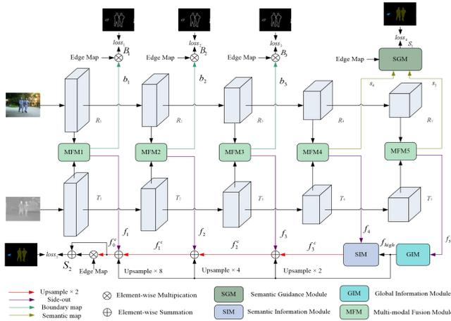
Figure 1: Architecture of proposed EGFNet for scene parsing.
