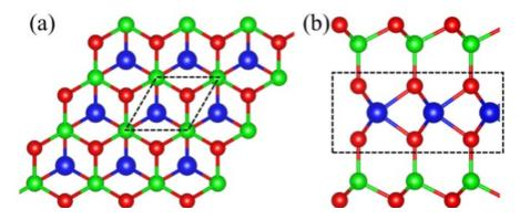
**FIG. 1** (a) Top and (b) side views of the relaxed structure of  $MA_2Z_4$ . The blue, red, and green balls represent the M, A, and Z atoms, respectively. The unit cell is marked by dashed lines in (a). The structure can be regarded as a  $MZ_2$  triple-layer (resembling 1H-phase MoS<sub>2</sub>; dashed rectangle in (b)) encapsulated by buckled AZ layers.
