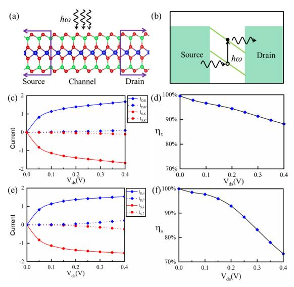
FIG. 6 (a)-(b) Schematic of the monolayer  $MA_2Z_4$  device and its generation of valley-polarized current. (c)-(f) valley currents, valley polarization, spin currents, and spin polarization of the monolayer  $MoSi_2P_4$  device.
