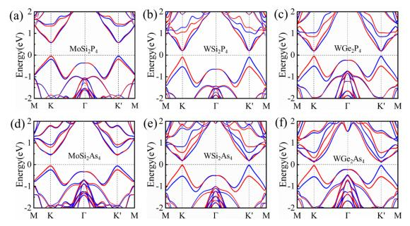
**FIG. 4** Band structures of monolayer MoSi<sub>2</sub>P<sub>4</sub>, WSi<sub>2</sub>P<sub>4</sub>, WGe<sub>2</sub>P<sub>4</sub>, MoSi<sub>2</sub>As<sub>4</sub>, WSi<sub>2</sub>As<sub>4</sub>, and WGe<sub>2</sub>As<sub>4</sub>. Red (blue) color represents dominance of the spin-up (spin-down) component.
