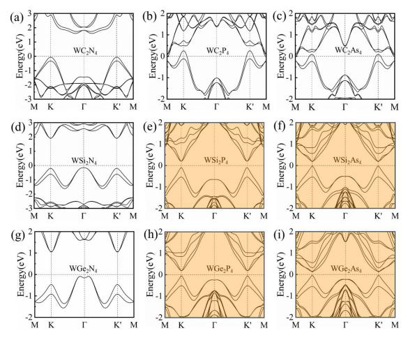
FIG. 3 (a)-(i) Band structures of monolayer  $WA_2X_4$ . The ones with the direct band gap are highlighted in orange.
