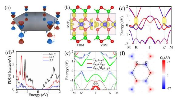
**FIG. 5** (a) Schematic of the valleys near the *K* and *K*' points, (b) charge densities at the VBM and CBM of MoSi<sub>2</sub>P<sub>4</sub>, (c) band structure of 1H-phase MoP<sub>2</sub>, (d) partial densities of states of MoSi<sub>2</sub>P<sub>4</sub>, (e) orbital-projected band structure of MoSi<sub>2</sub>P<sub>4</sub>, and (f) Berry curvature of MoSi<sub>2</sub>P<sub>4</sub>.
