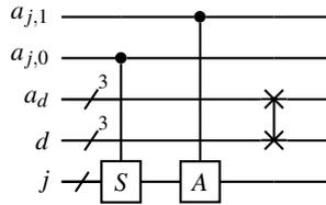
FIG. 13: Quantum circuit of the oracle  $O_M$ . The subtractor  $S$  and the adder  $A$  are shown in Fig. 14. The oracle converts the relative positions stored in the register  $|a_j\rangle$  into the corresponding absolute positions and stores them in the register  $|j\rangle$ . Then, the circuit swaps (Fig. 19) the registers  $|d\rangle$  and  $|a_d\rangle$ .
