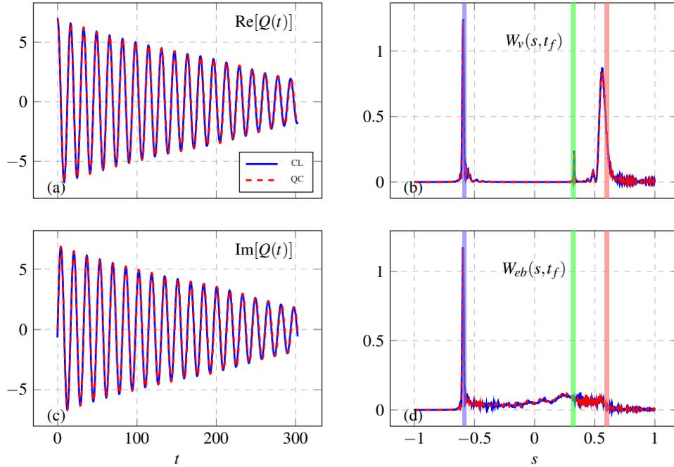
FIG. 16: Comparison of classical (solid blue curves) and emulated quantum (red dashed curves) simulations. Real (a) and imaginary (c) components of the source  $Q$ . (b): kinetic energy  $W_v$  (Eq. 11b) at time  $t_f$  as a function of  $s$ . (d): field energy  $W_{eb}$  (Eq. 11c) at time  $t_f$  as a function of  $s$ . The vertical lines show the HCR pair (blue), the LCR pair (green), the UHR (red).
