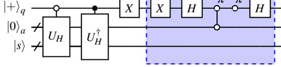
FIG. 7: Quantum circuit of the operator  $W$  (Eq. 31). The controlled unitary  $U_H$  (Eq. 24) and its complex-conjugate  $U_H^\dagger$  form the extended operator  $U'_H$  (Eq. 30). The left Pauli  $X$  gate implements the operator  $S$  (Eq. 29). The subcircuit within the blue box implements the reflector  $U_R$  (Eq. 32).
