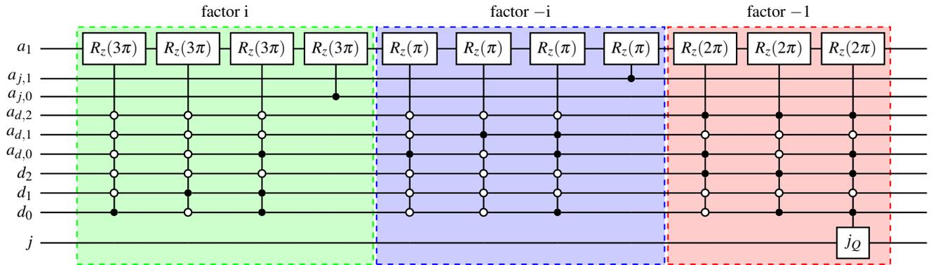
FIG. 12: Quantum circuit of the oracle  $O_{S, a_1}$ . The circuit is constructed according to Table III. Each colored box multiplies the amplitude stored in  $|a_1\rangle$  by the factor specified in the figure ( $i$ ,  $-i$ ,  $-1$ ). The rotation gate  $R_z$  acts as shown in Eq. 23.
