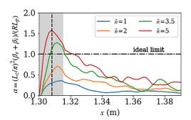
**FIG. 4.** Radial midplane profiles of  $\alpha=L_z^2\beta/(\pi^2RL_p)$ , the MHD ballooning stability parameter in helical geometry with no magnetic shear. The ideal ballooning limit  $\alpha = 1$  is shown as a dashed–dotted horizontal line.
