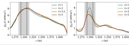
FIG. 5. Parallel heat flux to the lower endplate for ions (left) and electrons (right), computed via (18), normalized to the density scaling factor  $\hat{n}$ . There is a noticeable broadening of the electron heat flux profiles as  $\hat{n}$  increases with the peak flux about 25% lower in the  $\hat{n}=3.5$  and  $\hat{n}=5$  cases than the base ( $\hat{n}=1$ ) case. There is a little change in
