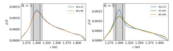
**FIG. 9.** Comparison of electron  $\beta$  profiles with low perpendicular resolution (16 × 32, blue) and high resolution (48 × 96, orange) for the  $\hat{n}=1$  (left) and  $\hat{n}=5$  (right) cases. While there is a little difference in the profile in the low-resolution  $\hat{n}=5$  case. Also included is an intermediate-resolution  $\hat{n}=5$  case (32 × 64, green) to verify numerical convergence.
