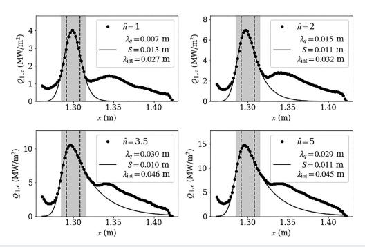
**FIG. 6.** Radial profiles of the electron parallel heat flux to the lower endplate for each case with the peaks fitted to (19). The heat-flux width  $\lambda_q$  increases by more than a factor of 4 between the  $\hat{n}=1$  and  $\hat{n}=3.5$  cases, which gives a quantitative measure of the turbulent broadening due to electromagnetic effects.
