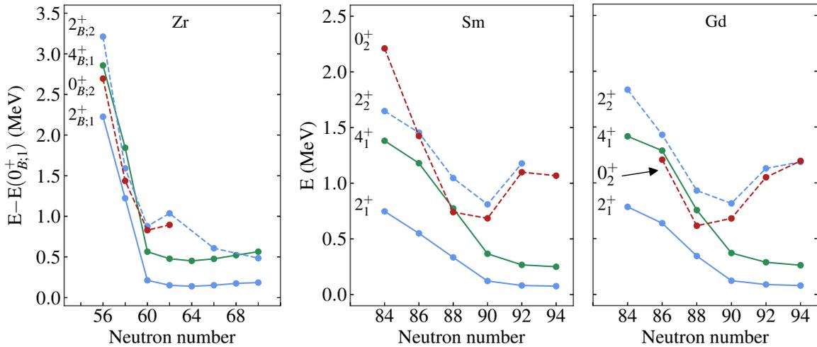
FIG. 15. Experimental energy levels in MeV, comparing the evolution with neutron number of states  $L_{B;i}^+$  of the  $B$  configuration in the Zr isotopes to the situation encountered in the Sm and Gd isotopes. Note that the energy of states in the  $B$  configuration of Zr are with respect to the lowest state ( $L = 0_{B;1}^+$ ) in that configuration. Data taken from [70].
