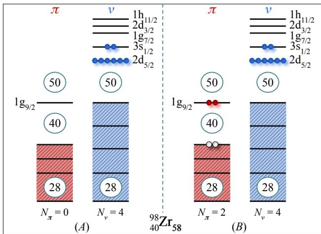
FIG. 2. Schematic representation of the two coexisting shell-model configurations ( $A$  and  $B$ ) for  ${}^{98}\text{Zr}_{58}$ . The corresponding numbers of proton bosons ( $N_\pi$ ) and neutron bosons ( $N_\nu$ ), relevant to the IBM-CM, are listed for each configuration.
