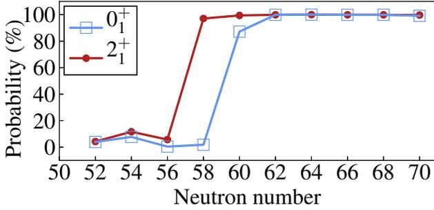
FIG. 10. Percentage of the wave functions within the intruder B-configuration [the  $b^2$  probability in Eq. (16)], for the ground ( $0_1^+$ ) and excited ( $2_1^+$ ) states in  $^{92-110}\text{Zr}$ .
