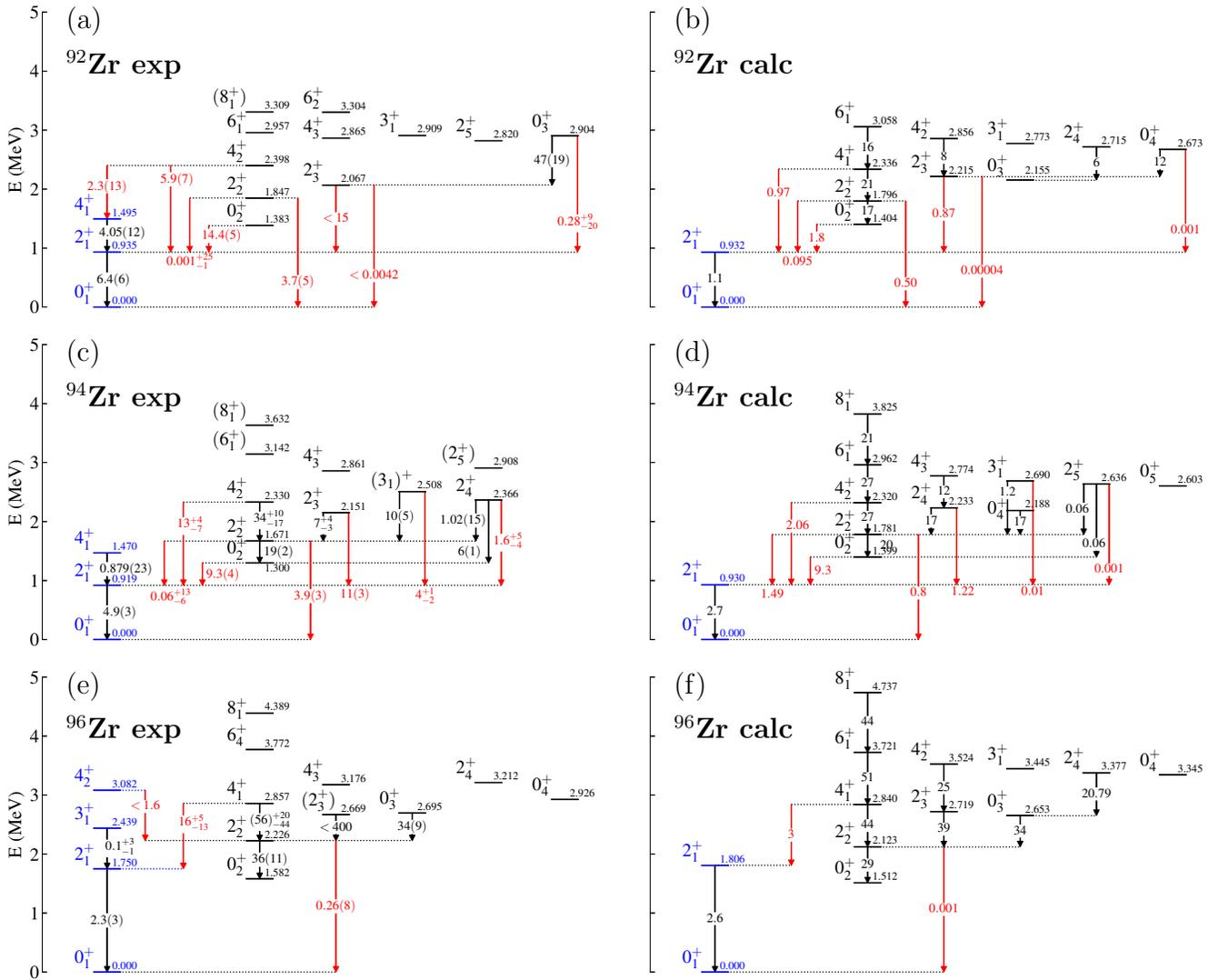
FIG. 4. Experimental and calculated energy levels in MeV and  $E2$  transition rates in W.u. Levels in blue (black) belong to the  $A$  ( $B$ ) configuration. Transitions between different configurations are denoted in red. For the configuration  $A$  experimental levels that have no corresponding calculated levels; see the Appendix. Data are taken from [53] for  $^{92}\text{Zr}$ , [25, 54] for  $^{94}\text{Zr}$ , and [28, 55] for  $^{96}\text{Zr}$ .
