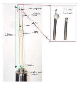
Figure 2. Photograph of the Langmuir probe with the different material tips. The zoomed-in area shows the burned probe tip after the experiment (left is tungsten and right is stainless steel).
