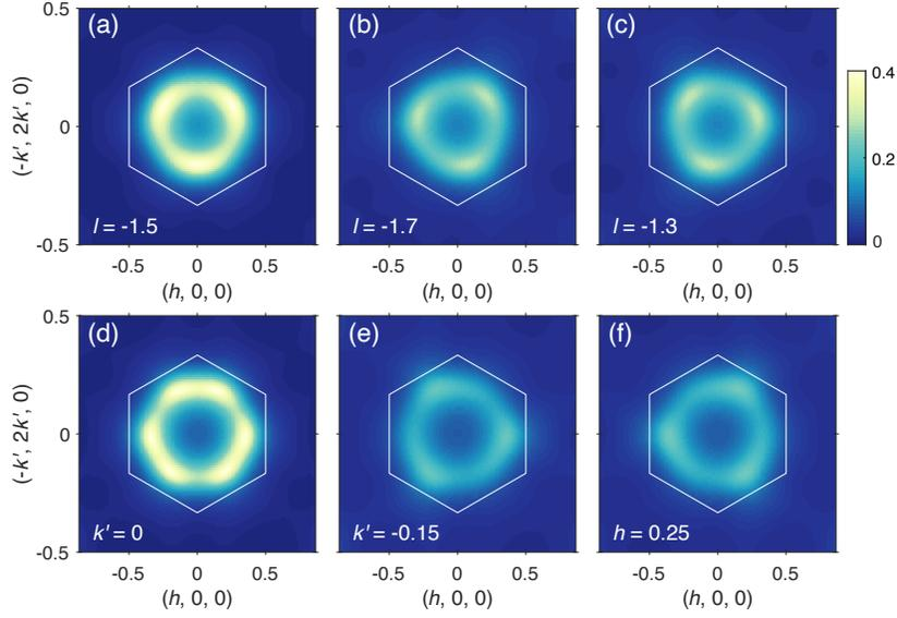
FIG. S6. Calculated diffuse scattering patterns for the  $J_1$ - $J_2$ - $J_{c1}$  minimal model being perturbed by the Kitaev couplings over the  $J_1$  bonds with (a-c)  $\phi = \pi/16$  and (d-f)  $\phi = -\pi/16$ . The calculation temperature is 10 K. The same color scheme is used for all the panels.
