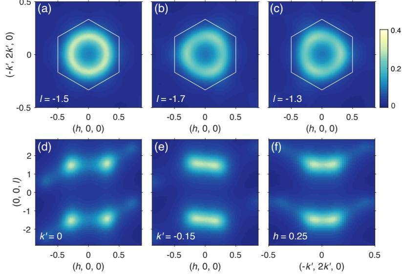
FIG. S5. Calculated diffuse scattering patterns for the  $J_1$ - $J_2$ - $J_{c1}$  minimal model at  $T = 10$  K with  $J_1 = -0.3$  meV,  $J_2 = 0.075$  meV, and  $J_{c1} = 0.15$  meV. The same color scheme is used for all the panels.
