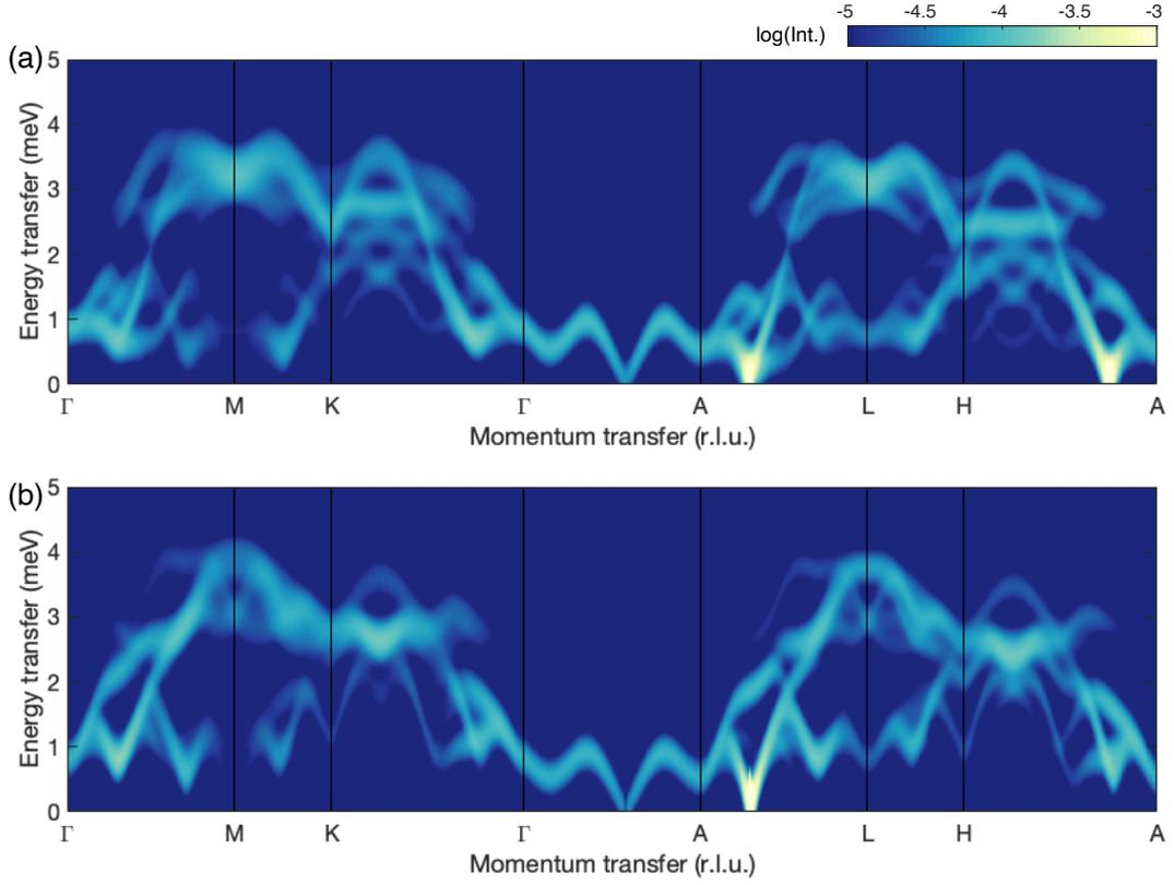
FIG. S8. Calculated INS spectra for the (a)  $J_1$ - $J_4$ - $J_{c1}$ - $J_{s1}$  and (b)  $J_1$ - $J_5$ - $J_{c1}$ - $J_{s1}$  models with coupling strengths shown in the text. For both calculations, a weak easy-plane single ion anisotropy of  $1 \mu\text{eV}$  is applied to stabilize the helical ground state.
