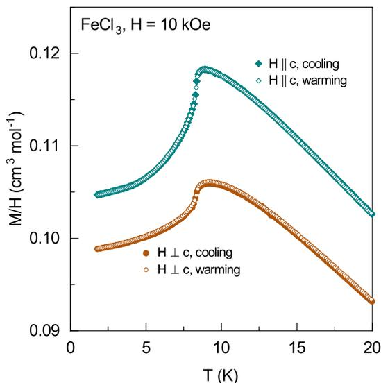
FIG. S1. Temperature dependence of the magnetic susceptibility ( $M/H$ ) measured with a field of 10 kOe applied in the plane ( $\perp c$ ) and out of the plane ( $\parallel c$ ) on cooling and subsequent warming.
