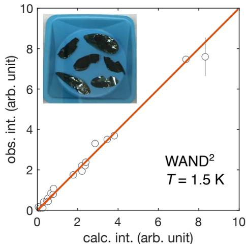
FIG. S2. Comparison between the calculated and observed intensities of the nuclear Bragg peaks collected at  $T = 1.5$  K. Inset is a picture of the  $\text{FeCl}_3$  crystals with a typical size of  $\sim 2.5$  cm in length and  $\sim 0.2$  cm in thickness. The weigh boat containing the crystals is 9 cm on a side and the photo was taken through the glove box window.
