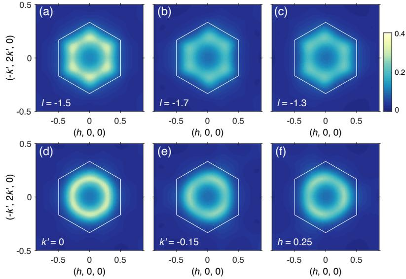
FIG. S7. Calculated diffuse scattering patterns for the  $J_1$ - $J_2$ - $J_{c1}$  minimal model being perturbed by the Dzyaloshinskii-Moriya interactions over the  $J_2$  bonds with the DM vectors along the  $c$  axis (a-c) and within the  $ab$  plane (d-f). The calculation temperature is 10 K. The same color scheme is used for all the panels.
