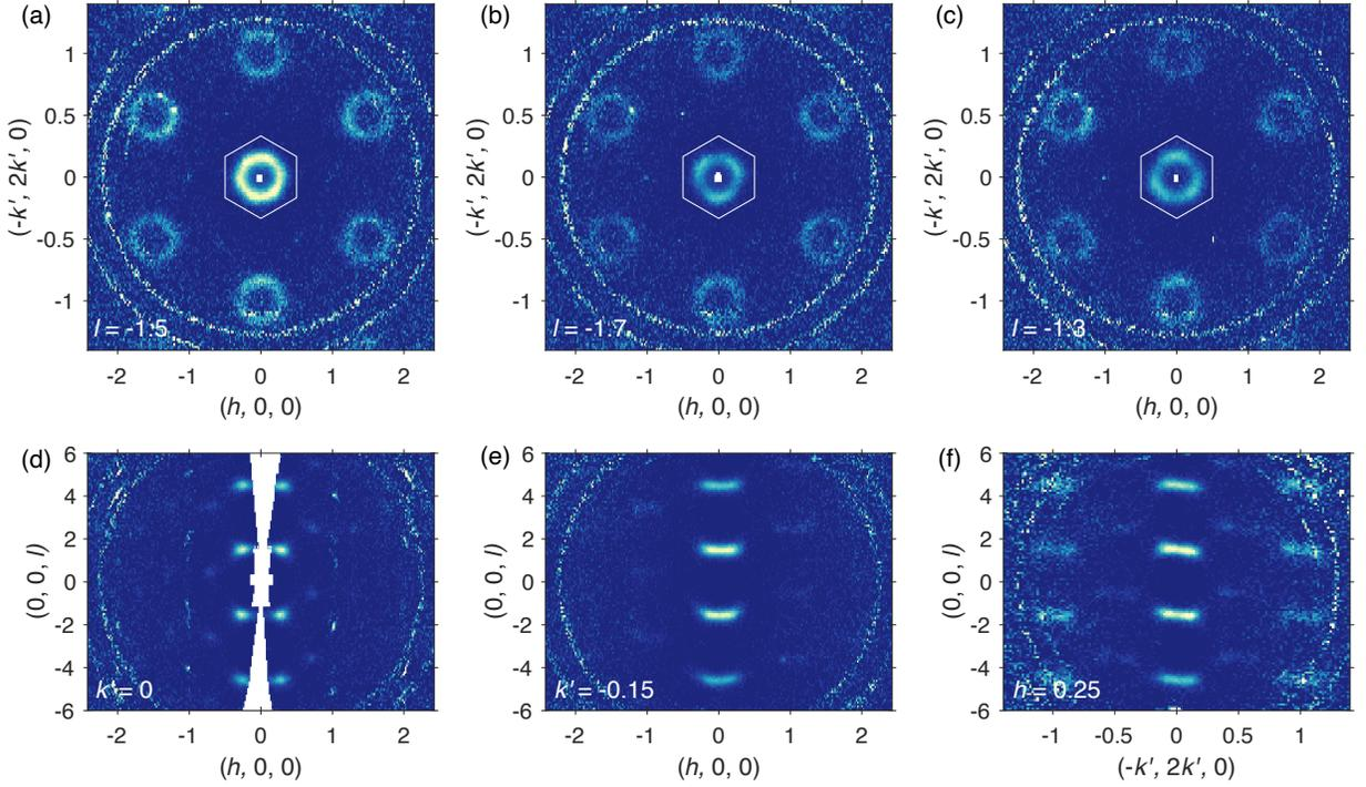
FIG. S4. Diffuse neutron scattering intensity measured at 10 K in a wide range. Data in the  $l = -1.5$ ,  $-1.7$ , and  $-1.3$  planes are shown in panels (a-c), respectively. Data in the  $k' = 0$ ,  $k' = -0.15$ , and  $h = 0.25$  planes are shown in panels (d-f), respectively.
