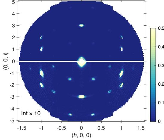
FIG. S3. Elastic slice of the SEQUOIA data in the  $k = 0$  plane collected at  $T = 4$  K with  $E_i = 8$  meV. The integration ranges are  $k = [-0.05, 0.05]$  r.l.u. and  $E = [-0.25, 0.25]$  meV. Data have been symmetrized according to the  $R\bar{3}$  space group symmetry. Intensity in the lower half panel is multiplied by 10 times to expose the weak streaks underneath the nuclear Bragg peaks.
