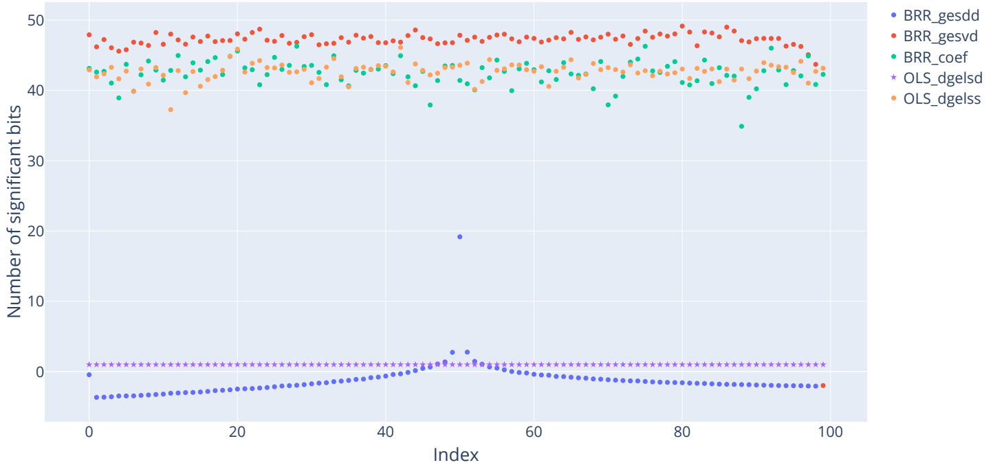
Figure 10: Precision of Bayesian Ridge Regression coefficients in RR mode. BRR_* show the BayesianRidge results using the gesdd and gesvd methods. OLS_* show the LinearRegression results with the dgelsd and dgelss methods. The Divide & Conquer method (gesdd and dgelsd) has low precision for BRR and results in NaN values (star points) for OLS. By switching to the gesvd method, results have a precision of 42 bits on average.
