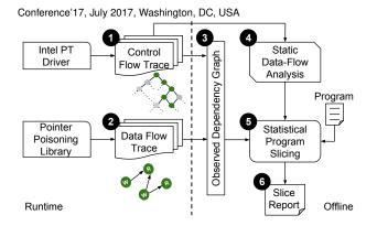
Figure 2: Overview of WOK's Architecture: runtime monitoring phase (left) and slice crafting phase (right).
