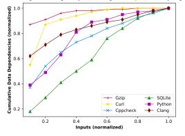
Figure 3: Cumulative distribution of data dependencies. Each cumulative distribution shows the fraction of the data dependencies recovered after each input. Each application runs against several thousands inputs.
