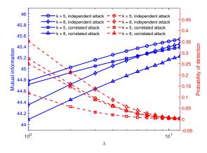
Fig. 8: Performance of attack constructions on IEEE 14-bus test system with  $\rho=0.9$ , SNR = 30dB and  $\tau=2$ .
