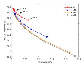
Fig. 3: Performance of independent sparse attack construction in terms of mutual information and KL divergence for different values of  $\lambda$  on the IEEE 9-bus system with SNR = 30 dB and  $\rho = 0.9$ .
