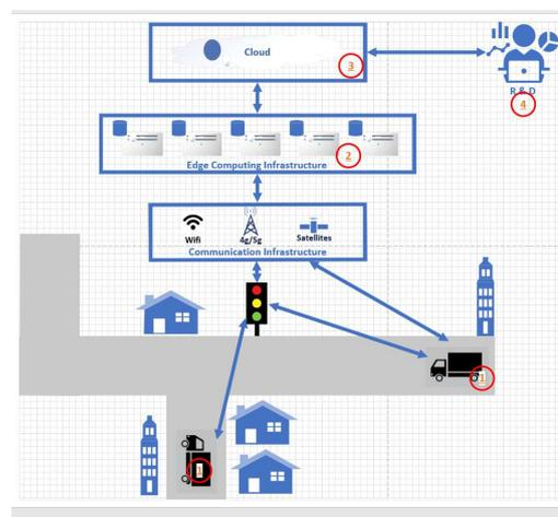
**Figure 1: Illustration of parts of an ITS; computational nodes are shown with markers: (1) automated vehicles, (2) local infrastructure, (3) cloud, and (4) developer/operator/maintainer center. Figure courtesy of Naveen Mohan, KTH.**
