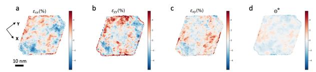
**Fig. 9.** Normal ( $\varepsilon_{xx}$  and  $\varepsilon_{yy}$ ) and shear ( $\varepsilon_{xy}$ ) strain maps of the Pd@Pt nanoparticle in **Fig. 6**.
