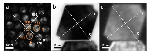
Fig. 6. Local coordinate system used for strain measurement. (a) Lattice vectors  $\vec{a}$  is from (000) disk to (111) disk and  $\vec{b}$  from (000) disk to (111) disk. The X-axis is along (000) to (220) and Y-axis along the (002). (b-c) The corresponding X and Y axes are marked in the BF and reconstructed ADF image.
