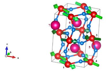
**Figure 1.** Electric dipole moments arrangement in RCrO<sub>3</sub> unit cell. Green arrows denote the orientation of electric dipole moments in the vicinity of  $Cr^{3+}$  ions ordered by antiferroelectric *D* mode.
