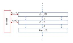
Fig. 2. Visual representation of the network, with *s* systems connected to the leader and the others connected through the *in-domain coupling*
