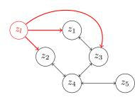
Fig. 1. Example of network considered in this paper: black connections represent the *in-domain* connection between the systems while red connections represents the systems who are communicating with the leader.
