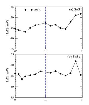
FIG. 7: (Colour online) Calculated values of  $|Im\Sigma(\omega)|$ along W-L- $\Gamma$  direction at 700 K for the top most VB of (a) SnS and (b) SnSe.
