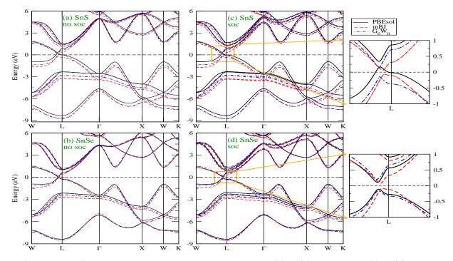
FIG. 1: (Colour online) Electronic band structures of SnS and SnSe (a) & (b) without and (c) & (d) with including spin-orbit coupling using PBEsol (black solid line), mBJ (red dashed line) and  $G_0W_0$  (blue dotted dash line).
