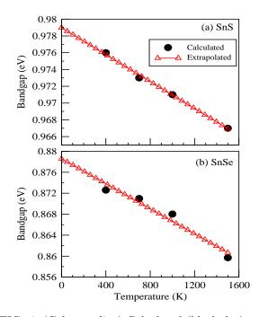
FIG. 4: (Colour online) Calculated (black dot) and extrapolated (red sold line) temperature dependent bandgap at L-point for (a) SnS and (b) SnSe.
