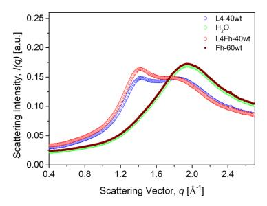
**Figure S1**. Wide-angle X-ray profiles in a linear-linear plot of the background ( $H_2O$ ), ferrihydrite dispersion diluted in  $H_2O$  to 60 wt.% (Fh-60wt), 40 wt.% lamellar phase in  $H_2O$  (L4-40wt) and 40 wt.% lamellar phase prepared using the ferrihydrite dispersion (L4Fh-40wt).
