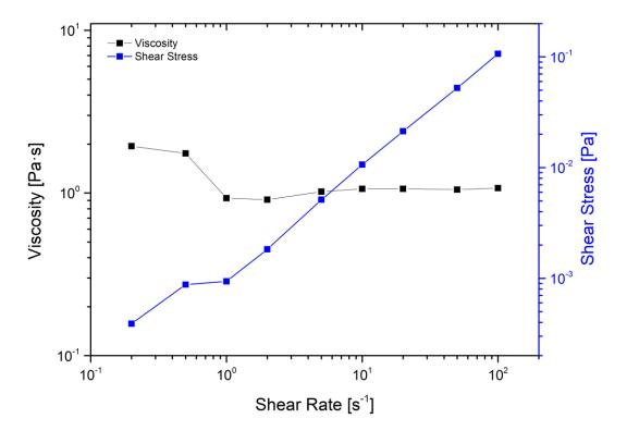
Figure S3. Steady-state viscosity and corresponding shear stress as a function of the shear rate for Ferrihydrate dispersion (Fh).
