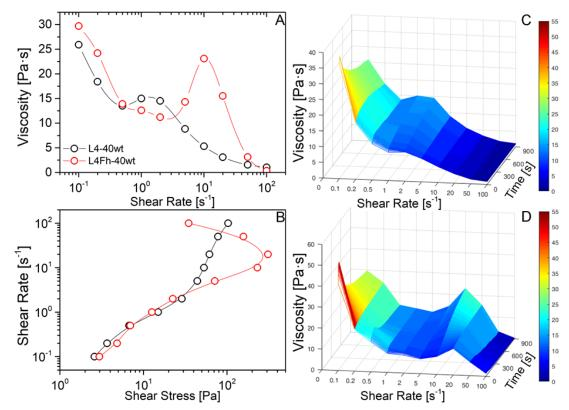
**Figure 2**. Steady-state viscosity as a function of the shear rate (A) and corresponding shear rateshear stress plot (B) for the 40 wt.% L4 lamellar phase (L4-40wt) and the 40 wt.% L4 lamellar phase prepared in the Fh dispersion (L4Fh-40wt). Three-dimensional plots of the transient experiments performed to obtain the steady-state values are reported for both the L4-40wt (C) and
