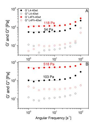
**Figure 3**. Frequency sweep measurements before (A) and after (B) applying a shear rate of 5 s<sup>-1</sup> to the 40 wt.% L4 lamellar phase (L4-40wt) and for the 40 wt.% L4 lamellar phase prepared in the Fh dispersion (L4Fh-40wt). The red and black lines are linear fitting of the data.
