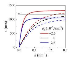
Fig. 3 (color online). The group velocity of spin waves inside wall (solid lines) and domain (dashed lines) of a FiM system for various  $\delta_s$ .
