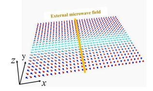
Fig. 1 (color online). Illustration of a FiM wall of the Bloch type. External microwave field is applied along the *x*-axis to excite the spin wave that propagates along the *x* direction too.
