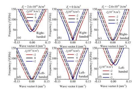
Fig. 4 (color online). Current-induced Doppler shift of right-handed spin waves in a FiM system for (a)  $\delta_s > 0$ , (b)  $\delta_s = 0$ , and (c)  $\delta_s < 0$ , and the shift of left-handed spin waves for (d)  $\delta_s > 0$ , (e)  $\delta_s = 0$ , and (f)  $\delta_s < 0$ .
