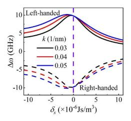
Fig. 5 (color online). Doppler shift for right- (dashed lines) and left-handed (solid lines) spin waves as a function of  $\delta_s$  for various wave vectors.
