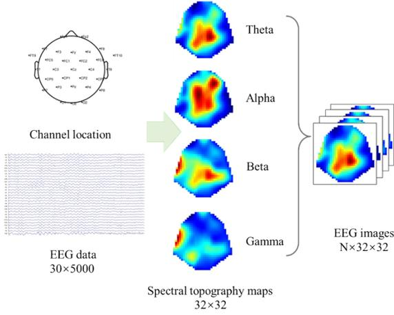
Figure 1. The method of 2D EEG image generating by EEG data
