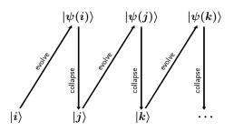
Figure 2. Schematic representation of the METTS algorithm whose procedure consists of the following steps: (i) choose a cps  $|i\rangle$ ; (ii) evolve it to a metts  $|\psi(i)\rangle$  in imaginary time according to Eq. (6) and calculate quantities of interest; (iii) collapse  $|\psi(i)\rangle$  into a new cps  $|j\rangle$  with the probability  $\mathcal{P}(i \rightarrow j) = |\langle j | \psi(i) \rangle|^2$  and then return to the step (ii).
