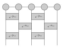
Figure 1. Diagrammatic representation of the TEBD algorithm for a quantum lattice system of 5 sites with nearestneighbor interactions. The full Hamiltonian is splitted into two parts,  $H = H_{odd} + H_{even}$  with  $H_{odd} = h_{1,2} + h_{3,4}$  and  $H_{even} = h_{2,3} + h_{4,5}$ . The odd and even numbered two-site local evolution operators are alternatively applied to the wave function represented by a matrix product state (MPS) [73].
