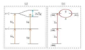
Fig. 1. (Color online) (a)Energy level diagram of conventional photon blockade realized by the system.(b)The photon state and interference path of non-traditional photon blockade are realized in the system.
