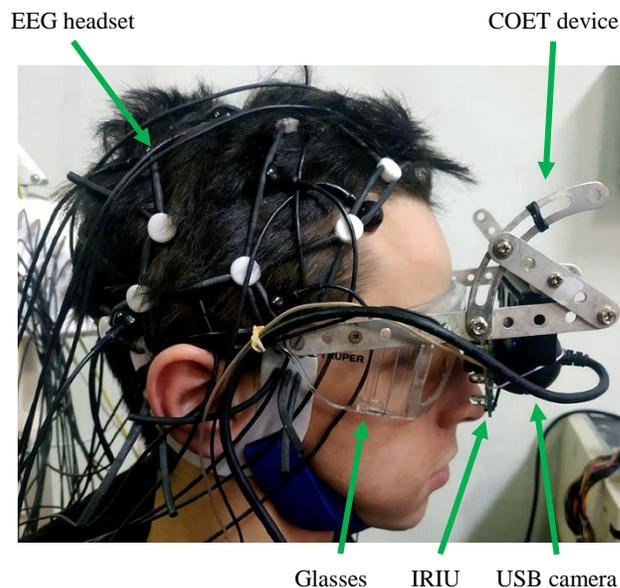
Fig. 2. Our experimental system on a test person.
