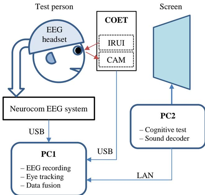
Fig. 1. Schematic representation of the developed experimental system.
