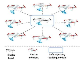
Fig. 2. UAVs' network architecture.
