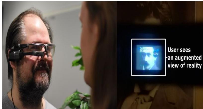
Figure 8.11. Face analysis with smart glasses. (© CMVS)
