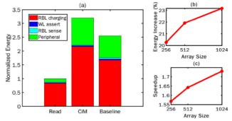
Figure 6: (a) energy components of read, ADRA based CiM and baseline, (b) energy decrease and (c) speedup of ADRA based CiM as a function of array size for precharged RBL voltage sensing (scheme 1)
