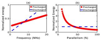
Figure 5: energy comparison for CiM using precharged (scheme 1) and discharged RBL (scheme 2) voltage sensing schemes as a (a) function of frequency of CiM operation and (b) parallelism of CiM operation
