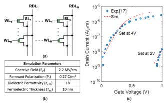
Figure 2: (a) 1T FeFET array, (b) simulation parameters and (c) I-V characteristics of the modelled device calibrated using the work in [17]
