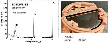
**Fig. 2.** *Left:* calibration of a 200 g Nb<sub>x</sub>Si<sub>1-x</sub> Ge bolometer using <sup>71</sup>Ge activation by neutrons. The Ge crystal was biased at 66 V for NTL amplification. *Right:* the top surface of the detector is covered by a TES layer and a 2 % coverage Al grid. The bottom Ge surface is fully covered by an Al grid. (Color online)
