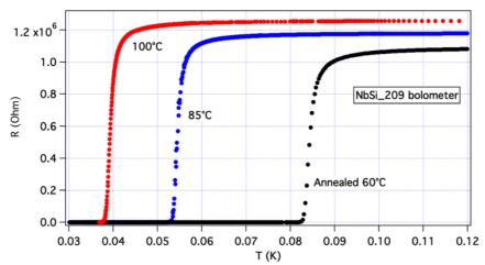
**Fig. 1** Annealing effect of a 100 nm thick Nb<sub>0,132</sub>Si<sub>0,868</sub> film deposited on a 200 g Ge crystal. The sample has been annealed three times during one hour at increasing temperatures. After each annealing, the superconducting transition curve is measured in a dilution refrigerator. This method allows to lower the TES critical temperature in a reproducible way. (Color figure online)
