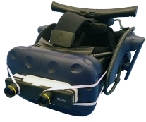
Fig. 3. A VR HMD with VST capabilities: the HTC Vive Pro with mounted Zed Mini camera
