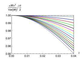
FIG. 2. Plot of the TUR ratio for the work done  $\left(\frac{\langle W \rangle^2}{\operatorname{Var}[W]}\right) / \left(\frac{\sigma}{2}\right)$  (array of dots) against the time duration  $\tau$ . The horizontal axis is measured in units of seconds. We changed the value of the spring constant from  $m\omega_0^2 = 10^{-8} \mathrm{Kg/s^2}$  (the top light blue) to  $m\omega_0^2 = 2.9 \times 10^{-7} \mathrm{Kg/s^2}$  (the down light blue).
